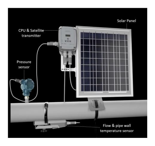
The primary mechanism for reading activity in the pipe is through the ultrasonic acoustic waves sent and received by the transducer. These waves are powerfully transmitted through the pipe wall, including any scaling or paraffin buildup and reflect off of the many bubbles or solids present in the flowstream.
